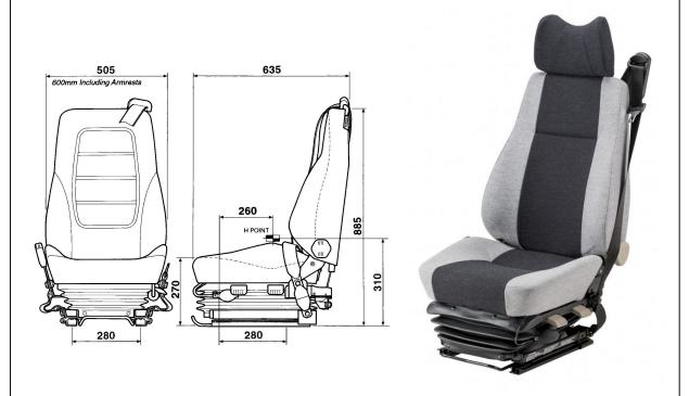
The KAB 714B is a self-levelling air suspension seat with double acting hydraulic damper incorporating a 3-point seat belt.
